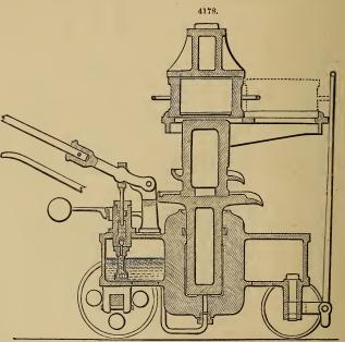
whole is about 16 cwt.; it will give a pressure of about 60 tons, and, with one press-box, will press about  $1\frac{1}{2}$  bushel of seed an hour.
